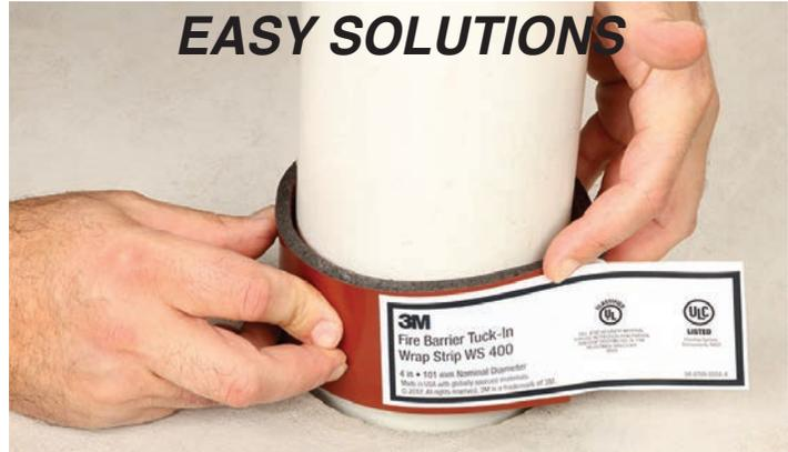
Intumescent wrap strip primarily used in top-side firestop installations. Available as precut strips for 2-inch, 3-inch or 4-inch plastic pipes and as an 8 foot roll which can be cut to length for larger plastic piping penetrations.
